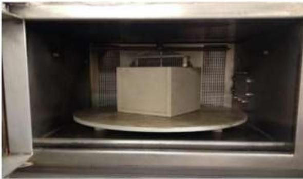
4 Photo of 100 mm concrete cube cast in PEREK mould in microw
