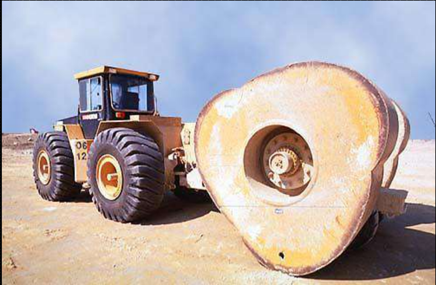
Impact Roller to Compact the Ground
