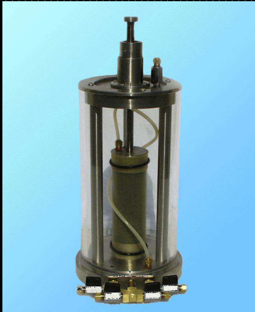
Triaxial Test on Soil Sample in Laboratory
