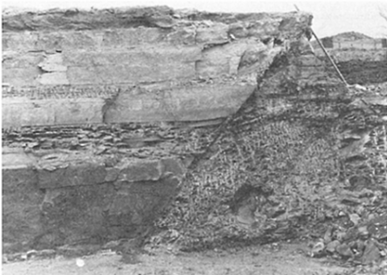
Figure 4.20 A small normal fault affecting Coal Measures (sandstone and shales) revealed in an excavation in Central Scotland. The sense of
