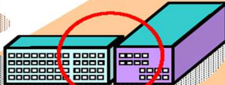
(c) Separation joints make complex plans into simple plans
