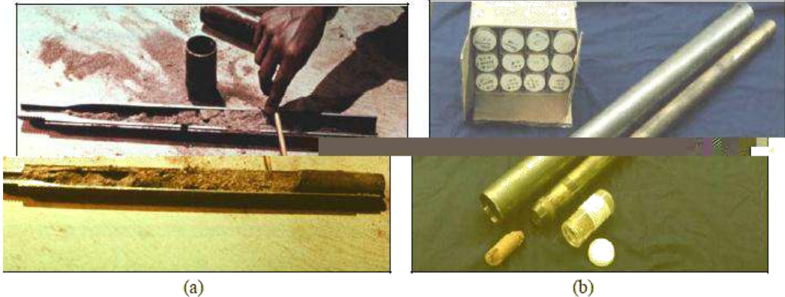
Split Barrel Sampler: (a) Open sampler with soil sample and cutting shoe; (b) Sample jar, split-spoon, shelly tube, and storage box for transport of jar samples.
