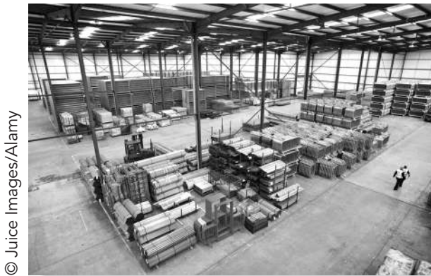
The design of the floor system of this warehouse building must account for critical locations of storage materials on the floor. Influence lines must be used for this purpose. (Photo courtesy of Portland Cement Association.)
