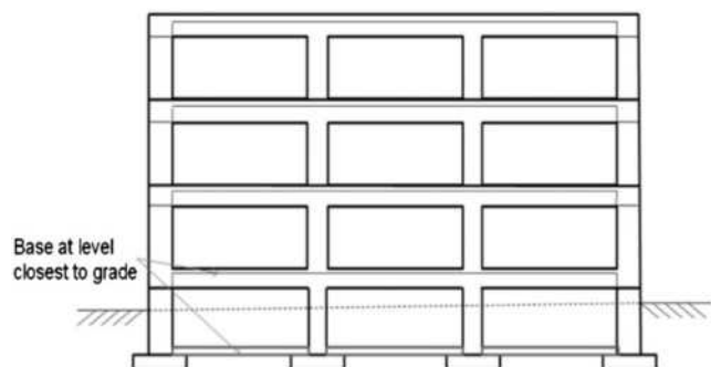
FIGURE C11.2-4 Base at Level Closest to Grade Elevation
