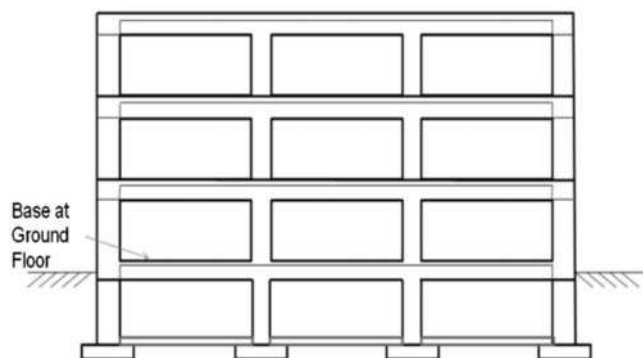
FIGURE C11.2-3 Base at Ground Floor Level
