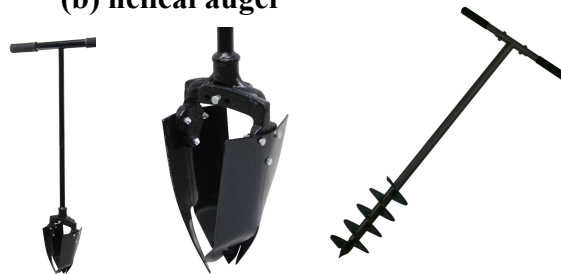
Hand tools: (a) posthole auger; (b) helical auger
