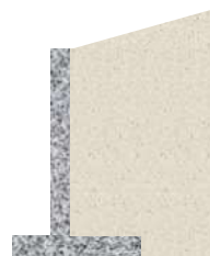
Cantilever retaining wall
