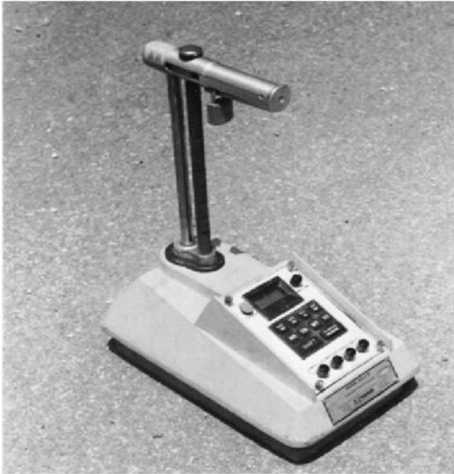
Figure 6.25 Nuclear density meter (Courtesy of Braja M. Das, Henderson, Nevada)
