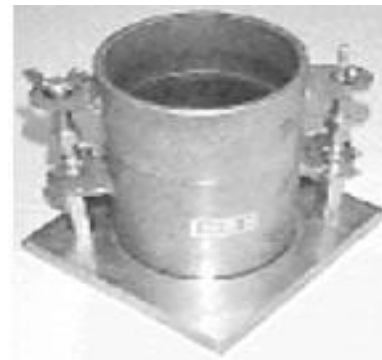
944 ml compaction mould
