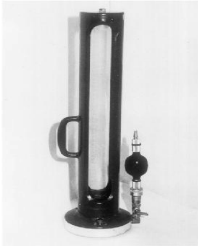
Figure 6.24 Calibrated vessel used with rubber balloon (not shown) (Courtesy of John Hester, Carterville, Illinois)
