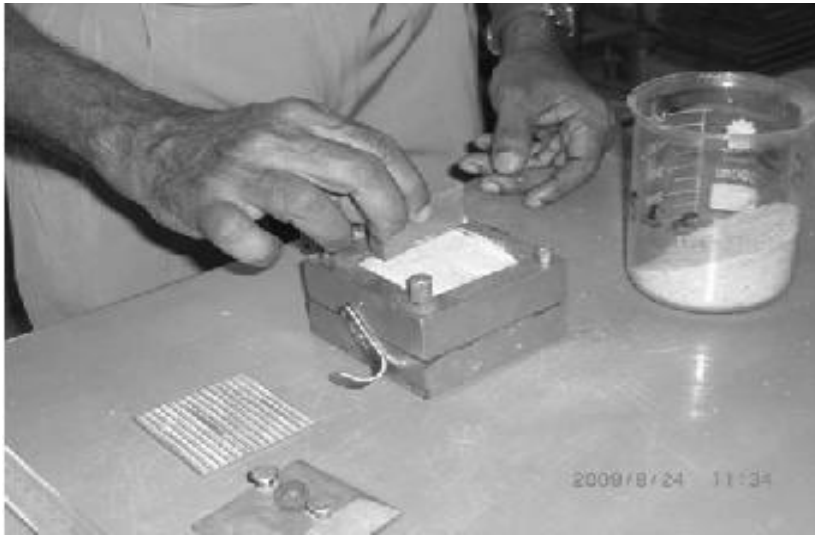
Leveling the top surface of specimen
