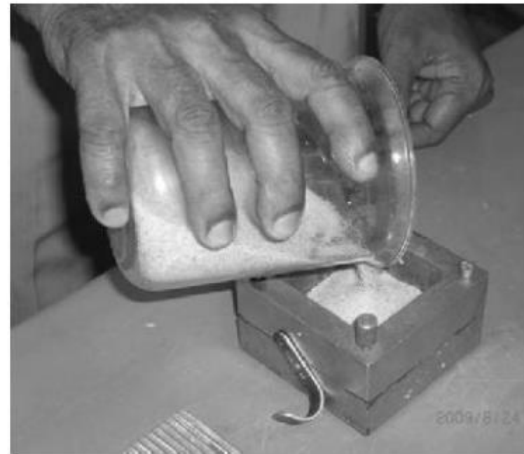
Preparation of a sand specimen
