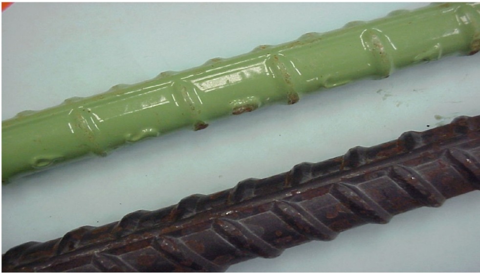
Special coatings are applied to steel, such as galvanizing or epoxy coating (green bar above) to protect against the exposure to salts in sea water.
