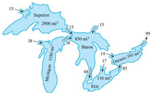
Figure 5.54 Compartmental model of the Great Lakes with flow rates ( \text{mi}^3/\text{yr} ) and volumes ( \text{mi}^3 )
