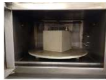
A Piece of 100 mm concrete cube cast in PESTE mould is shown
