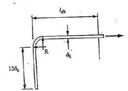
$\phi 10$  to  $\phi 25$ : R = 3d<sub>b</sub>  $\phi 28$  to  $\phi 32$ : R = 4d<sub>b</sub>  $\phi 50$ : R = 5d<sub>b</sub>.
