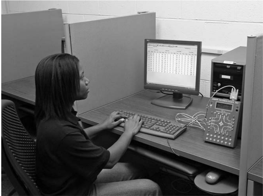
Figure 4.7 Jamar Traffic Data Collector TDC-12 Hooked to a Computer
