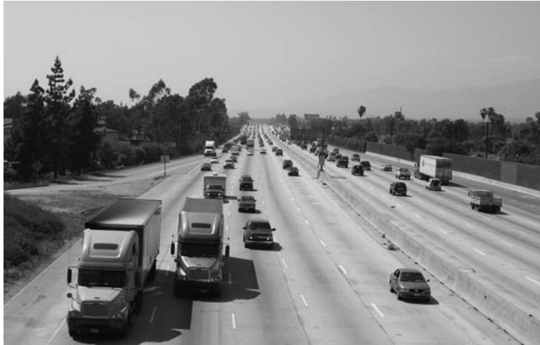
(a) Note the formation of large gaps in front of slow-moving trucks climbing the upgrade.
