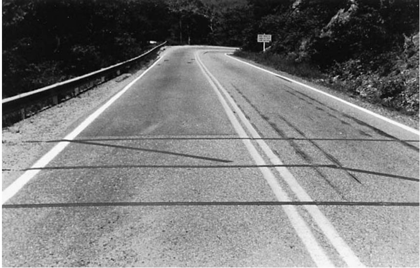
Figure 4.8 An Example of a Sensor Setup of a Surface Detector Using Pneumatic Road Tubes
