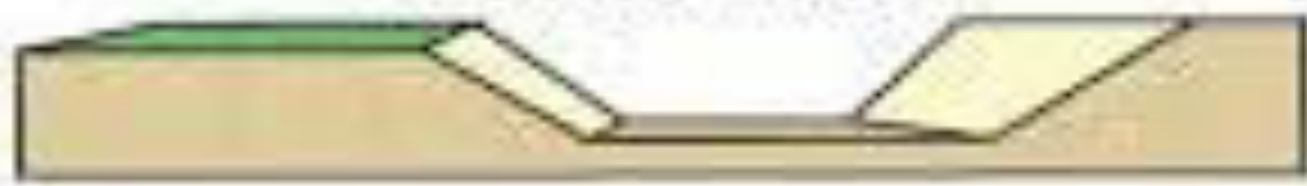
FLAT BOTTOM DITCH
