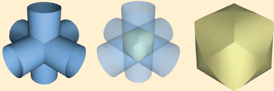
1. Sketch carefully the solid enclosed by the three cylinders  $x^2 + y^2 = 1$ ,  $x^2 + z^2 = 1$ , and  $y^2 + z^2 = 1$ . Indicate the positions of the coordinate axes and label the faces with the equations of the corresponding cylinders.
